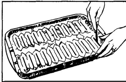
You can use aluminum foil to line your broiler pan and broiler rack. However, you must mold the foil tightly to the rack and cut slits in it just like the rack.
