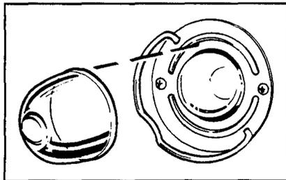
The oven lamp (bulb) is covered with a removable glass cover which is held in place with a bail-shaped wire. Remove oven door, if desired, to reach cover easily.
