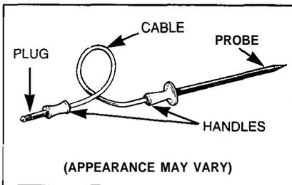
The temperature probe has a skewer-like probe at one end and a plug at the other end that goes into a receptacle on the oven wall. Use handles of the probe and plug when inserting and removing from meat and wall receptacle. Do not use tongs to pull on the cable when removing the probe—they might damage it. **TO AVOID BREAKING THE PROBE, MAKE SURE FOOD IS COMPLETELY DEFROSTED BEFORE INSERTING.**
