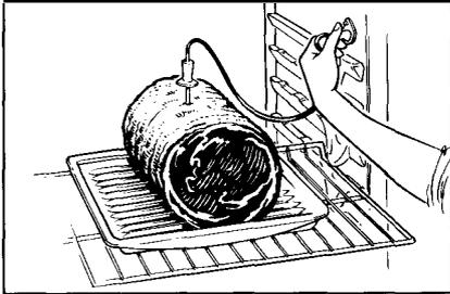
**Step 2:** Plug probe into receptacle on the oven wall. Make sure it's pushed all the way in. Close the oven door.
