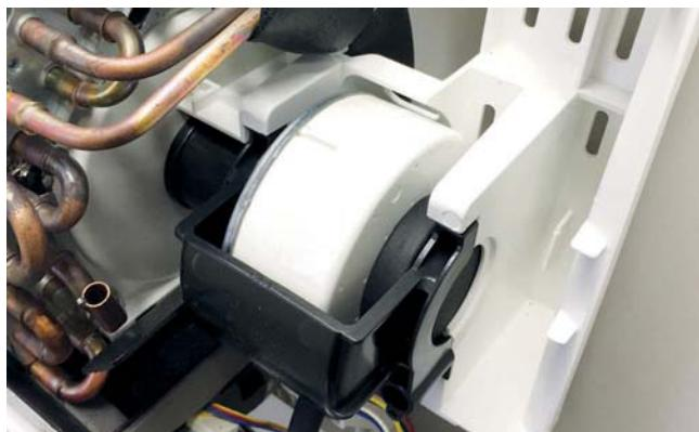
The Fan Motor is a variable speed DC motor. The motor will vary speed with the speed of the compressor. It will operate automatically or at a preselected fixed speed. When in AUTO fan mode, the speed of the fan is calculated using the difference between the set and room temperatures.
