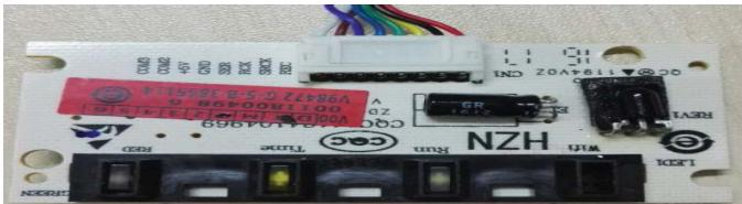
The indoor display is an infrared communication circuit that receives operating commands from the remote control. This display will indicate operating modes, error codes, indoor air temperature, timer and power status.
