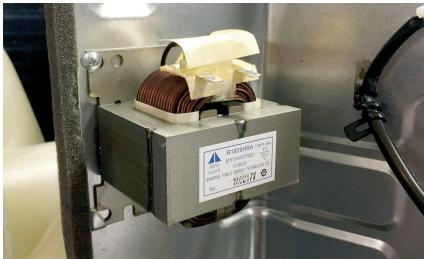
The Reactor is a power filter. It is unlikely to ever have an electrical failure of this component.
