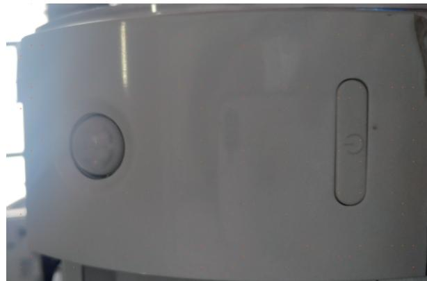
If the remote control is non-functional, the Emergency Button can be used. 73 -78 degrees will be maintained, until commands are received via the remote control.
