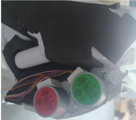
The STEPPER MOTOR moves the louver up and down, or right and left, depending upon selections made at the remote control.
