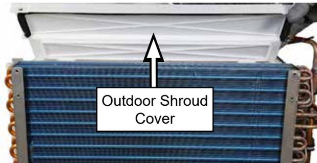
5. Remove two 1/4-in. screws from the base of the fan shroud. They are located on the right and left side.
