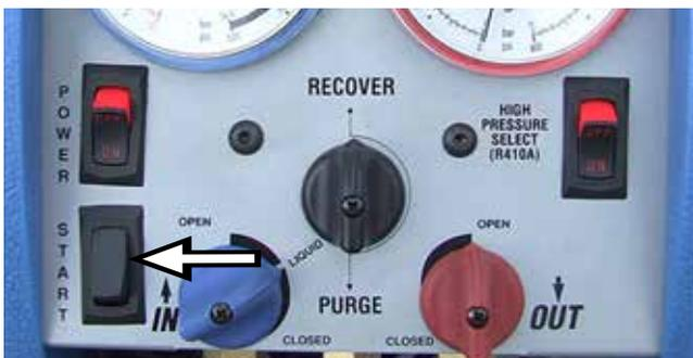
4. Throttle the output valve so that the output pressure is 100 psi greater than the input pressure, but not more than 300 psi.
