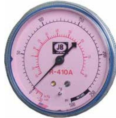
The inner dial of the high side pressure gauge reads the temperature in °F from 0 to 160.
