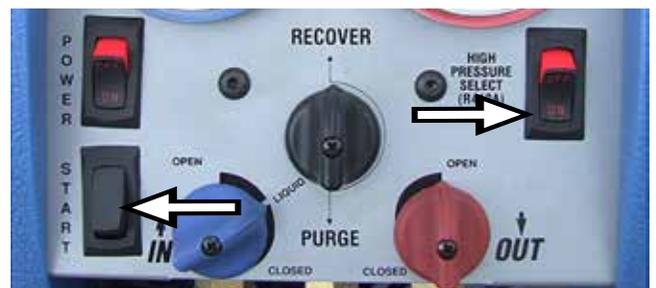
**NOTE:** If the pump begins to knock, slowly throttle back the input valve until the knocking stops.
