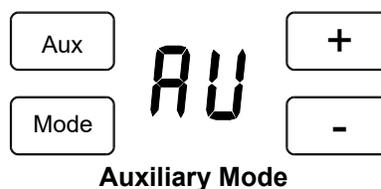
While in AUX Mode, press the **MODE** button to scroll through the eight different modes. Continue to press the **MODE** button until the number corresponding to the mode to be modified is showing in the first digit of the display. Once the correct number is displayed, use the **+/-** buttons to change the second digit of the display for that mode to either "Π" for **On** OR "⊥" for **Off** depending on the desired function.
