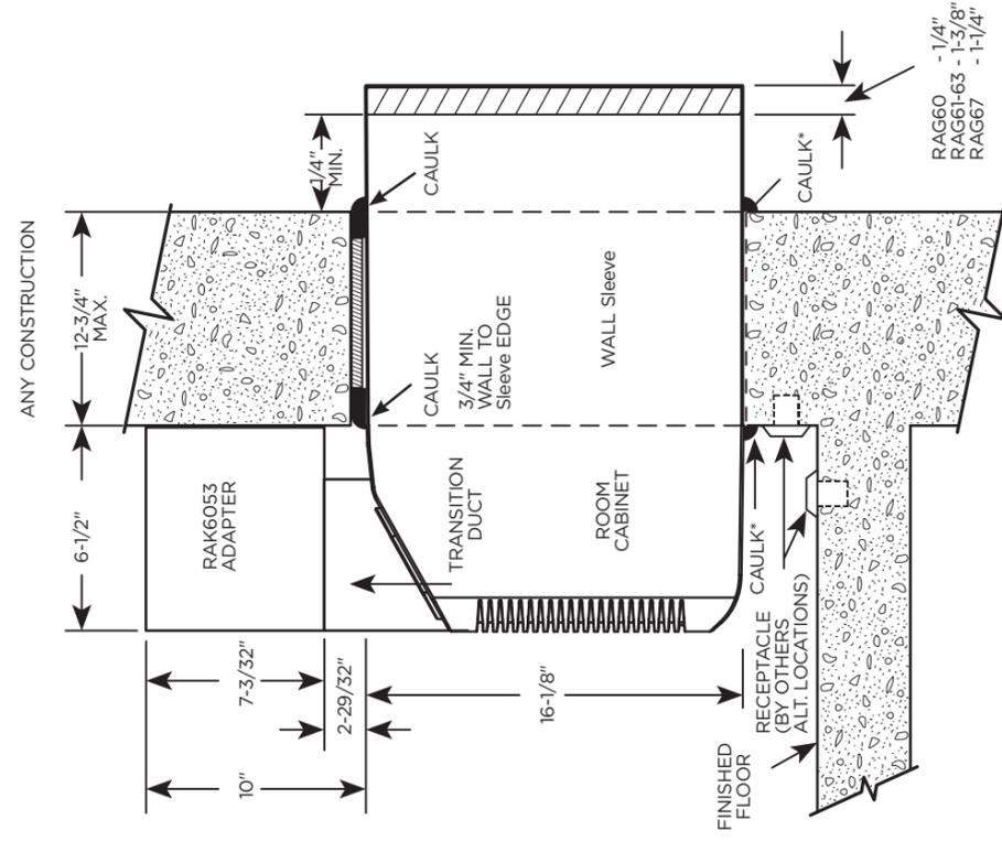
\*Caulk around perimeter of wall sleeve all four sides where it joins the building - Interior and Exterior.
