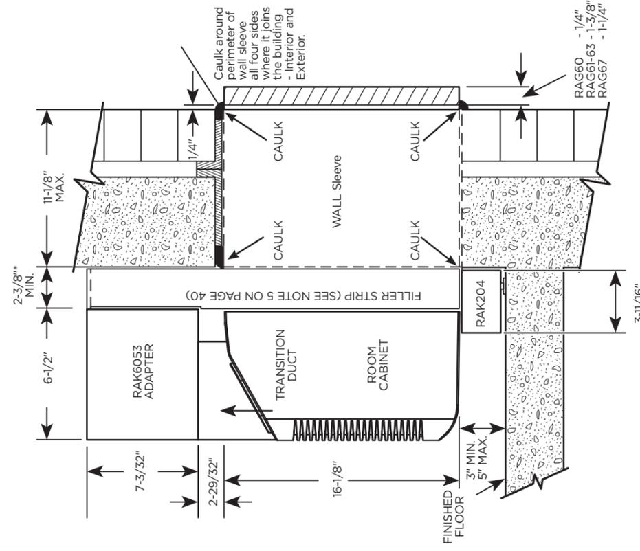
\*2-3/8" min. when installed with RAK204.
