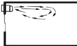
**High Wall Mount:** For units mounted high in the wall, the discharge louvers should be at a setting that provides the most horizontal air discharge. Recommended installation is at least 3" below the ceiling.
