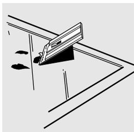
Using a razor scraper will not damage the surface if the 45° angle is maintained.
