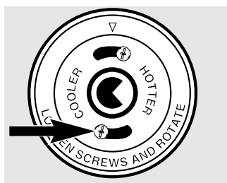
The lower screw moves toward COOLER to decrease the temperature.
