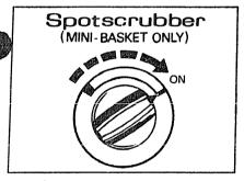
—Set SPOTSCRUBBER control to ON position. This fills the Mini-Basket tub half full of water which is normal!\*
