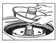
5. After loading clothes in the Mini-Basket tub, be sure to replace the Filter-Flo pan. The pan serves as a lid to keep the clothes in the Mini-Basket tub.
