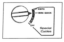
2. Push the Cycle Selector knob in and turn it clockwise to the MINI-QUICK Cycle.
