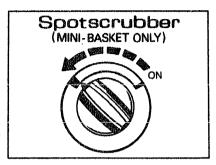
When agitation begins, the SPOTSCRUBBER control moves counterclockwise for about half a minute. A sharp distinctive sound will be heard soon after agitation begins. This is the sound of the water recirculation system cutting off to keep the concentrated detergent solution in the Mini-Basket tub. When agitation stops, the SPOTSCRUBBER control moves the remaining distance to the left and rinsing begins.
