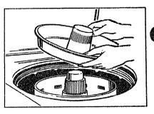
5. Replace the Filter-Flo pan. The pan serves as a lid to keep the clothes in the Mini-Basket tub.
