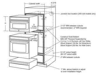
A=Allow 1" overlap of oven over top and bottom edges of cutout. B=Allow 11/16"-3/4" for overlap of oven over side edges of cutout.
