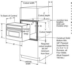
Note: Cabinets installed adjacent to wall ovens must have an adhesion spec of at least 194°F temperature rating.
