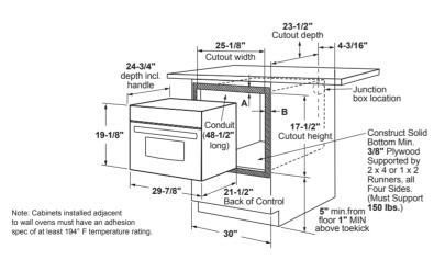
A= Allow 1" overlap of oven over bottom edge of cutout, and allow 1-1/4" overlap at top edge of cutout.
