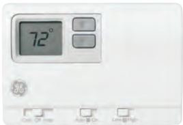
RAK148F2 HEAT PUMP DIGITAL TWO-FAN-SPEED THERMOSTAT • Two fan speeds • 24 VAC digital remote wall thermostat with single-stage cooling and 2-stage heating for heat pump models • Requires 7-wire hookup
