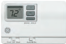
RAK164P2 COOLING WITH ELECTRIC HEAT PROGRAMMABLE REMOTE THERMOSTAT • 24 VAC programmable remote wall thermostat with single-stage cooling and single-stage heating for resistance heat models • Programmable for 7-day or 5+2-day programs • Requires 5-wire hookup
