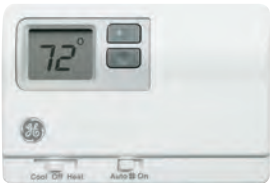
RAK148D2 HEAT PUMP DIGITAL REMOTE THERMOSTAT • 24 VAC digital remote wall thermostat with single-stage cooling and 2-stage heating for heat pump models • Requires 6-wire hookup
