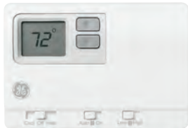
RAK164F2 COOLING WITH ELECTRIC HEAT DIGITAL TWO-FAN-SPEED THERMOSTAT • Two fan speeds • 24 VAC digital remote wall thermostat with single-stage cooling and single-stage heating for resistance heat models • Requires 6-wire hookup
