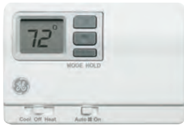
RAK148P2 HEAT PUMP PROGRAMMABLE REMOTE THERMOSTAT • 24 VAC programmable remote wall thermostat with single-stage cooling and 2-stage heating for heat pump models • Programmable for 7-day or 5+2-day programs • Requires 6-wire hookup
