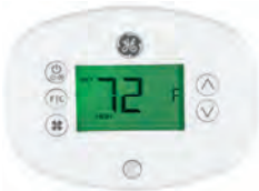
RAK180W1 HEAT/COOL ENERGY MANAGEMENT THERMOSTAT-UNIVERSAL/HEAT PUMP THERMOSTAT • 24 VAC • Wired (2-wire) or wireless (battery) • Occupancy detection for Energy Management and MUA control • Compatible for cooling with electric heat or heat pump Zoneline models • Customizable energy setbacks • Plug-and-play installation • Works with all Zonelines
