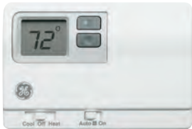
RAK164D2 COOLING WITH ELECTRIC HEAT DIGITAL REMOTE THERMOSTAT • 24 VAC digital remote wall thermostat with single-stage cooling and single-stage heating for resistance heat models • Requires 5-wire hookup
