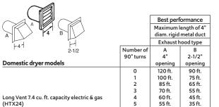
For every extra 90° elbow, reduce the allowable vent system length by 10 ft
