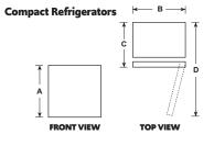
The unit should be placed with a 2" air clearance at the back wall and side walls and a 1/2" air clearance at the top.
