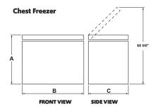
The unit should be placed with a 2" air clearance at the back wall and side walls.
