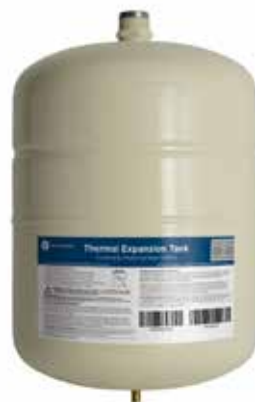
PM77X001 2.1 Gallon Expansion Tank • Connection Size: 3/4" Male Pipe Thread • Factory Pre-Charged: 40 PSI (2.8 bar) • Maximum air charge: 80 PSI (5.5 bar) • Maximum working pressure: 150 PSI (10.3 bar) • Maximum Temperature 200°F (93°C) • UPC Certified
