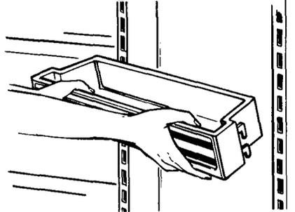
**To remove bins:** Lift bin straight up until mounting hooks disengage.
