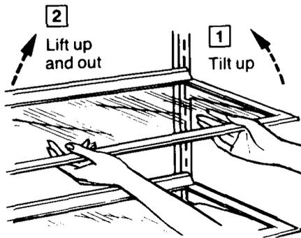
**To remove shelves:** Tilt shelf up at front, then lift it up and out of tracks on rear wall of refrigerator.
