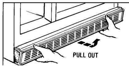
**To adjust rollers,** remove the base grille by grasping it at the bottom and pulling it out.
