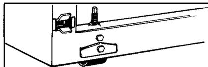
**When adjusting front rollers** for proper door closure, we recommend that the bottom front edge of the cabinet be approximately 3/4" from the floor.
