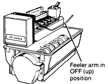
When water supply has been connected to icemaker, move feeler arm to ON (down) position.
