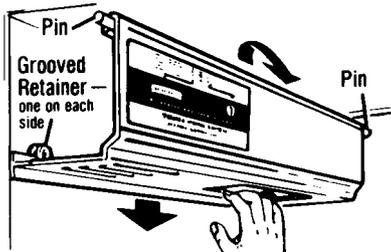
3. Pull bottom of light panel down about 1/4"—just enough to disengage lip at rear from grooves in retainers on rear wall.
