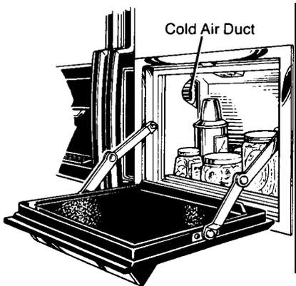
Cold air entering from the freezer compartment keeps the temperature in the Counter maker Compartment at proper food-keeping levels.
