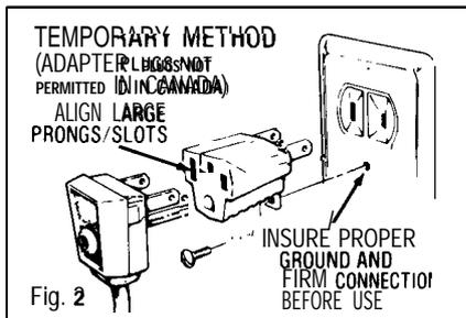
The larger slot in the adapter must be aligned with the larger slot in the wall outlet to provide proper polarity in the connection of the power cord.
