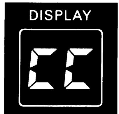
This flashing code tells you to **check temperature controls** and adjust them if necessary. (See directions on page 5.) Touch STATUS CHECK-RESET pad to erase code. If code reappears after 4 hours, call for service.
