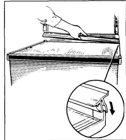
When drawers and covers are back in place, reinstall the gasket at the rear of the Sealed and Fresh drawer. Fit the end of the plastic drawer support into the slot on the gasket, with the rubber gasket flap facing you. Make sure the gasket snaps into place.
