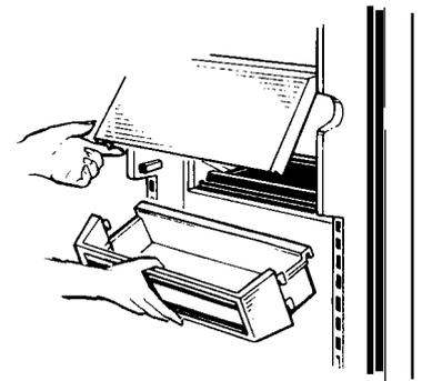
Then raise the inner door and lift the bin straight up until hooks on bin come out of tracks on door.
