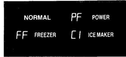
The word NORMAL is lighted except when a failure has been detected.
