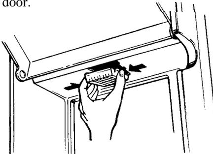
3. Press sides of flexible light shield to release locking tabs and allow the shield to swing down.
