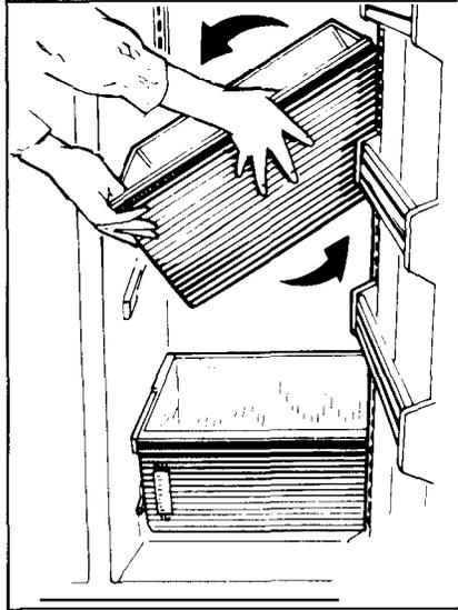
5. Pull the drawer forward, lift the front to clear stops, and remove the drawer. If the refrigerator door doesn't open completely, pull the drawer out until it hits the door. Then lift the drawer up until it is higher than the drawer supports, tilt it and take it out.
