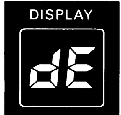
This flashing code tells you something's wrong with the defrost system—**keep doors closed to retain cold and call for service.** Code flashes until problem is corrected.
