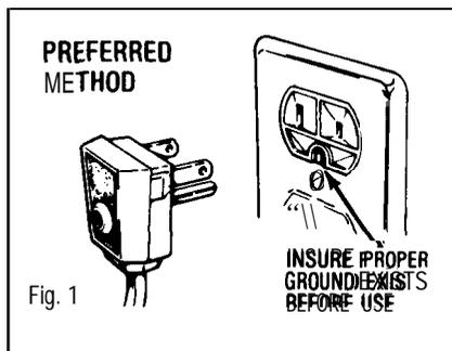
Have the wall outlet checked by a qualified electrician to make sure the outlet is properly grounded.
