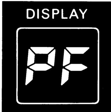
**This flashing code tells you the power to the refrigerator has been interrupted** for more than 2 seconds. Check the condition of food in both the fresh food and freezer compartments. Touch STATUS CHECK-RESET pad to erase code.
