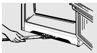
Cleaning the condenser coils.
